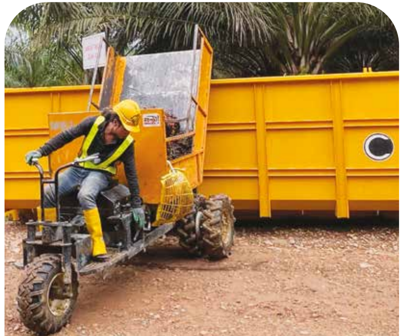
An estate worker in Air Puteh Estate operating a Mechanical Buffalo to transfer FFB.
