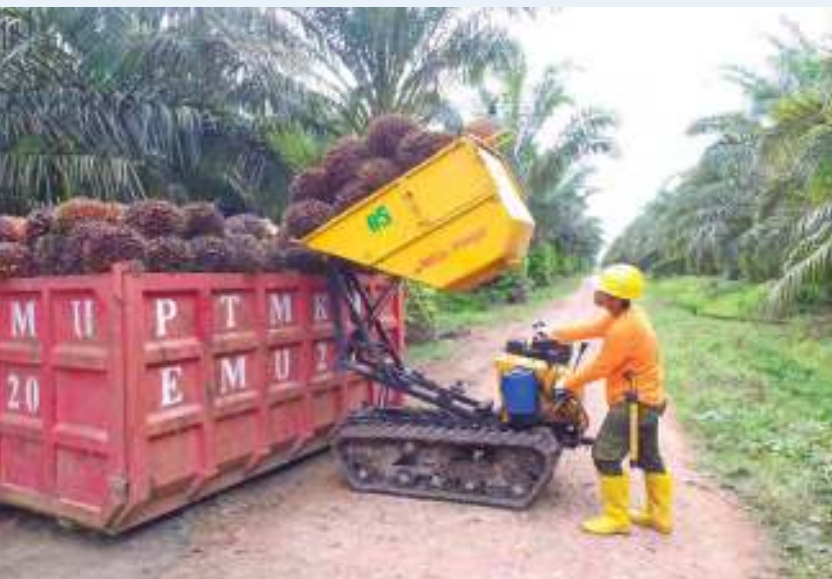
Harvesters using powered wheelbarrow to transfer ripe fresh fruit bunches into large bins to be transported to the mill
