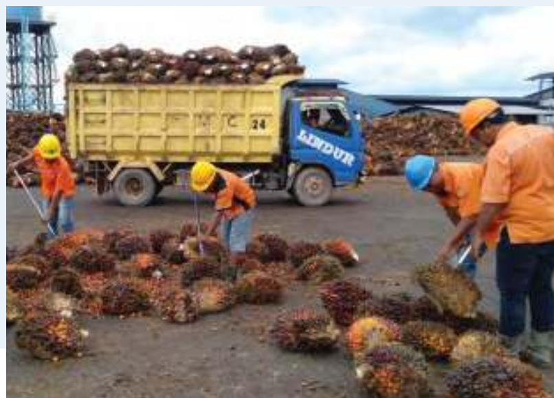
Each batch of fresh fruit bunches that arrived at the CPO mill are graded by mill workers to determine the quality of the harvested crop
