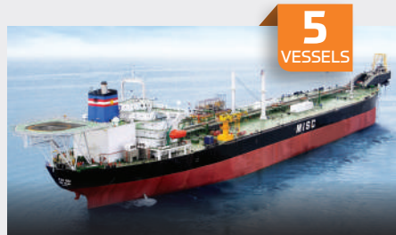
FLOATING STORAGE AND OFFLOADING (FSO)
