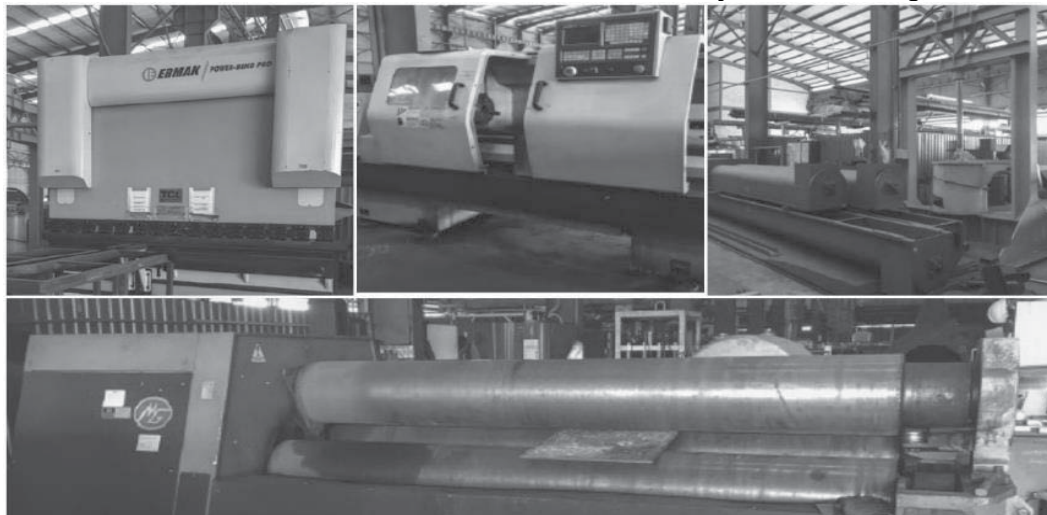
Top L to R: Bending machine; Computer numerical control (CNC) machining equipment; Shearing machine. Bottom: Rolling machine
