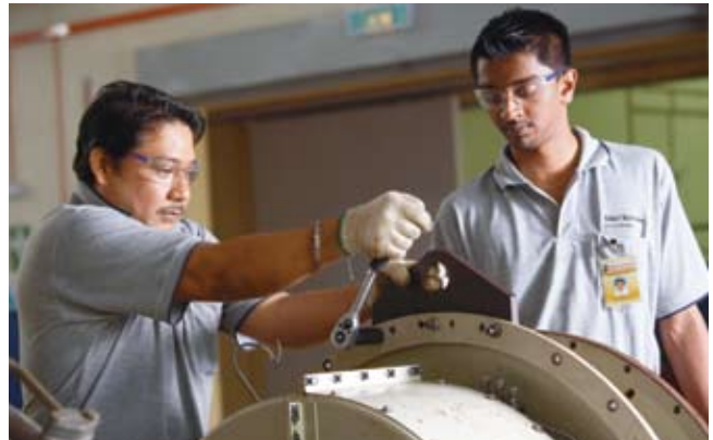
Turbine assembly works
