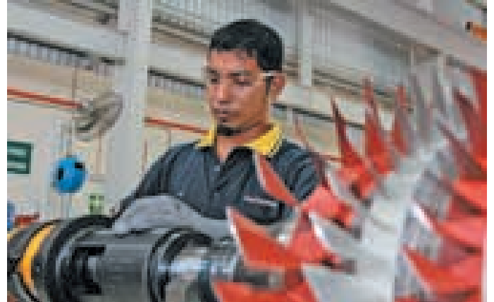
Overhaul of gas turbine
