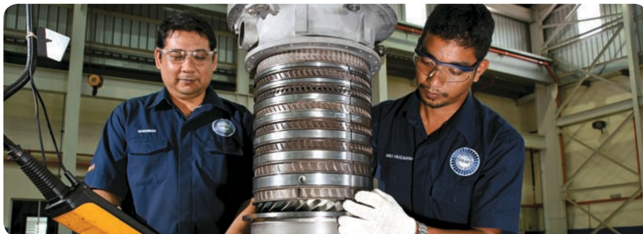
Gas Turbine assembly
