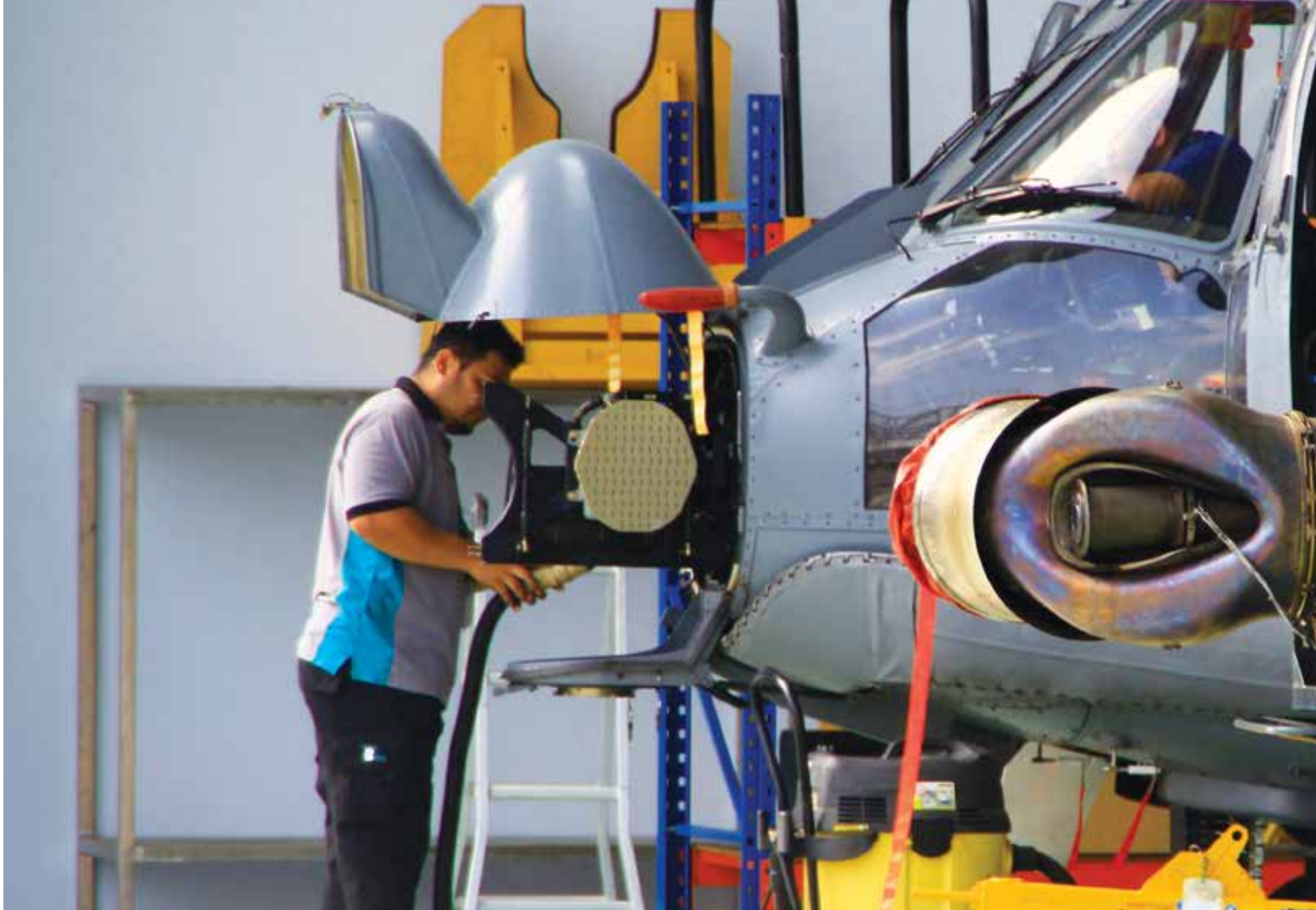
Inspection and functional test being carried out on the weather radar of an EC725 helicopter belonging to RMAF at BHICAS facilities
