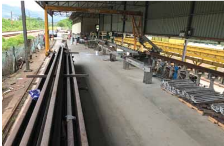
Production of Glued Insulated Rail Joints for Gemas-JB Double Tracking Project
