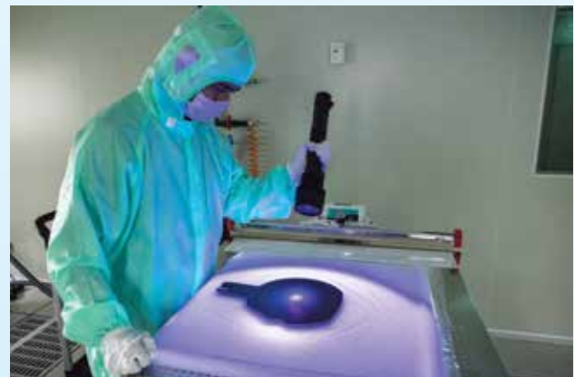
An employee performing visual inspection using Black Light (Ultraviolet) before final packaging process to confirm that there are no fibres/substrate microcracks.
