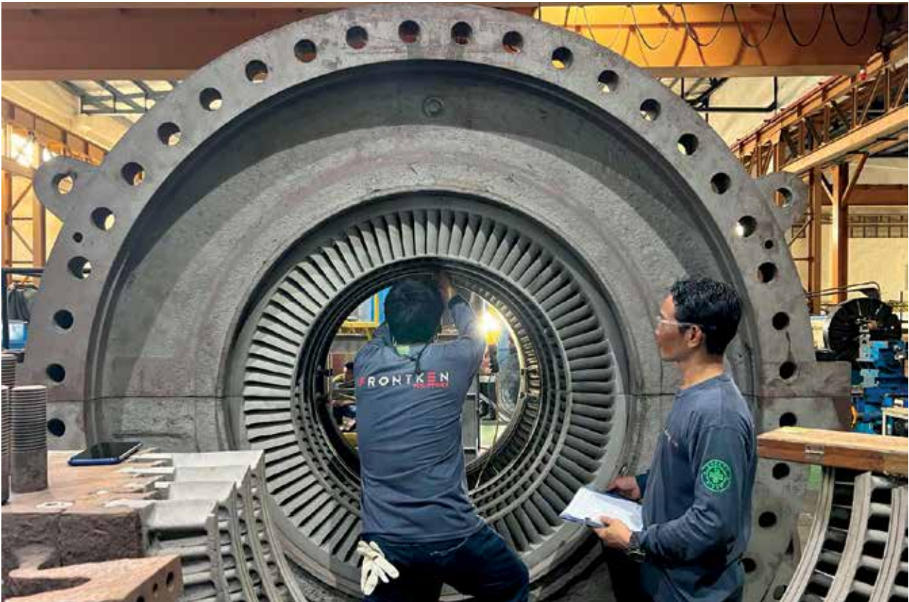
Palinpinon HP Diaphragm Repair
