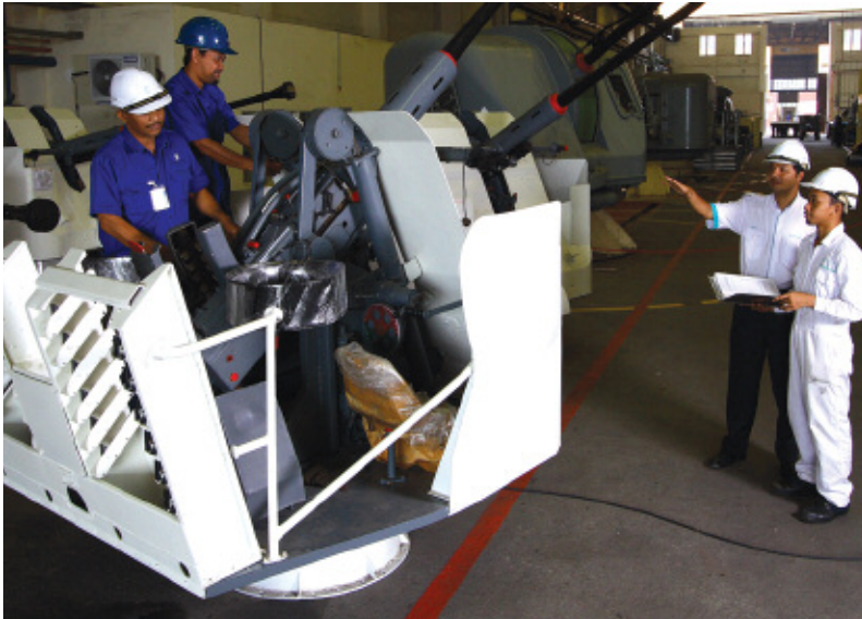
Weaponry experts repairing BOFORS guns at Lumut Yard.
