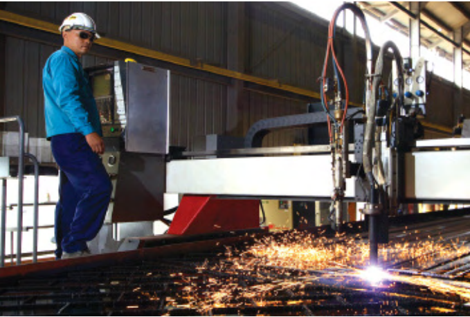
Our worker operating the computer numerical control (CNC) plate cutting machine at Jerejak Yard.
